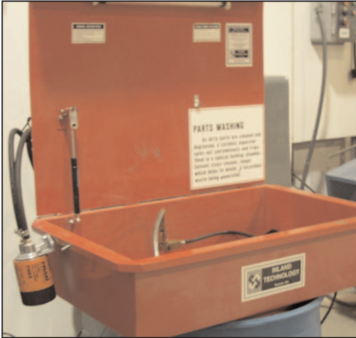
The oil filter installed on the parts washer
