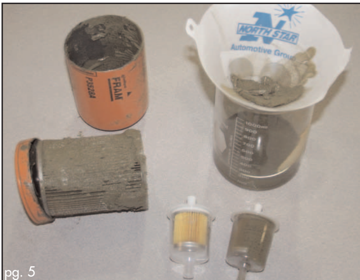
Cutting open the filter reveals that it really was working.
