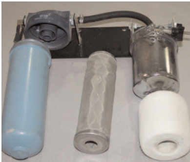
A typical add-on filtration unit
