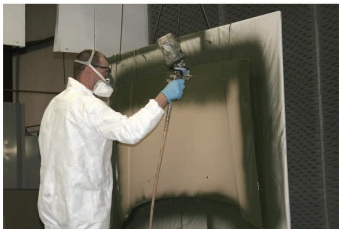
**Figure 3. A Military Technician Practices Proper Spray Technique on the Hood of a Vehicle.**
