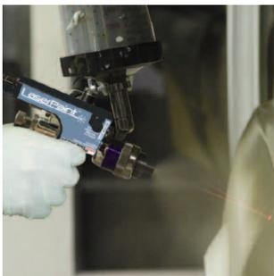
**Figure 2. Two Laser Beams Help the Coating Applicator Maintain Proper Distance from the Substrate and Keep the Coating on Target.**
