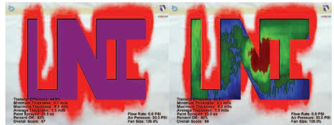
**Figure 5. Two Viewing Modes of the Virtual Training System: Single Color Mode (Left) and Accumulation Mode (Right). Various Thickness Levels Are Visible in the Accumulation Mode.**
